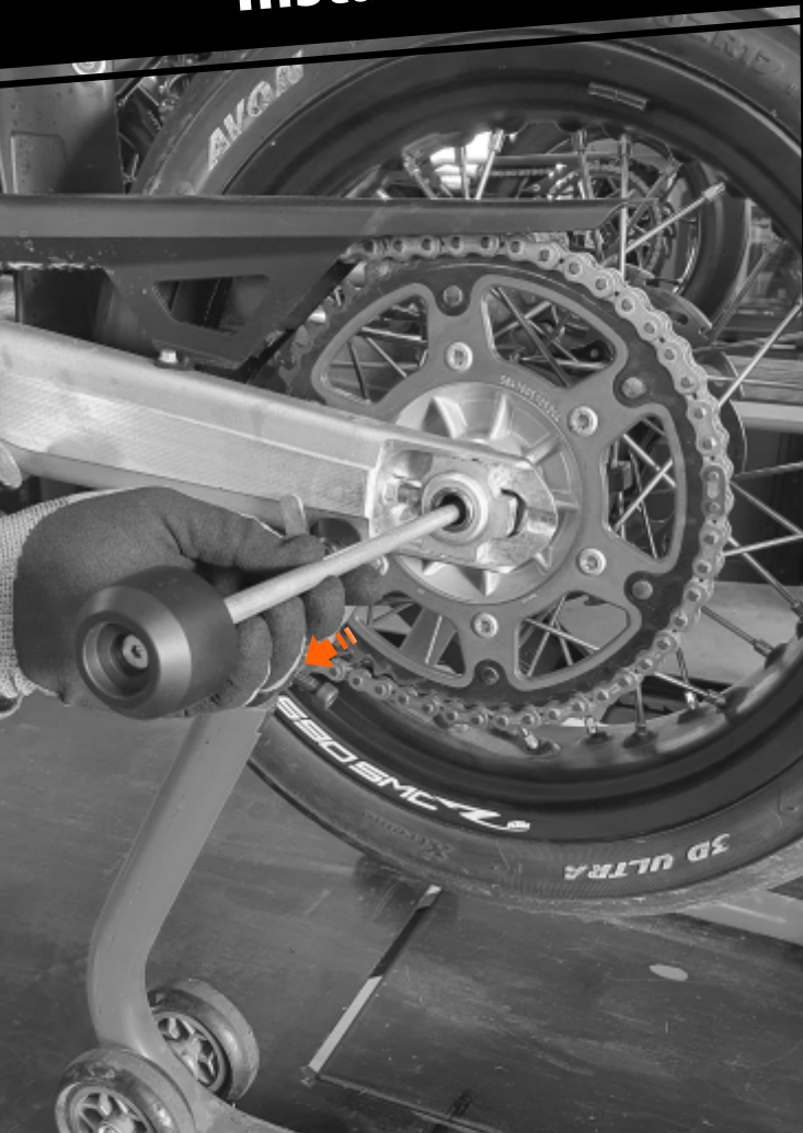
1. Slide the axle rod trough.
