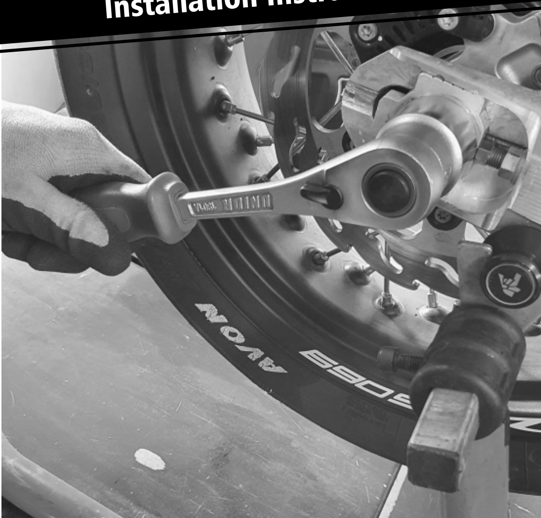
1. Fully tighten to max 6Nm.
