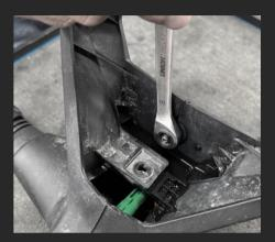
For turn signal nuts, use the supplied KTM spark plug socket wrench. Mark the position of the turn signals (left right) disconnect all connectors and remove the lights.
