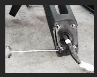
Unscrew the 2 signal light bolts and turn them to remove. Mark the position of the turn signals (left right) disconnect all connectors and remove the lights from the assembly
